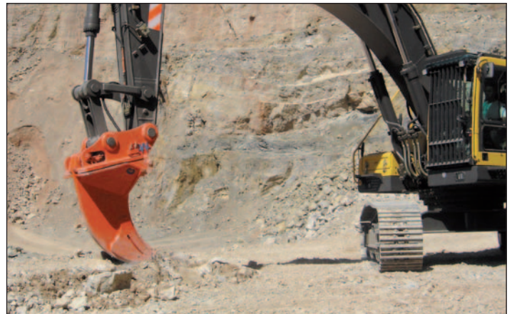
Rock ripper XXHD for extreme conditions, made from WHD 450 special wear steel, exchangeable protective shroud and tooth from Esco
