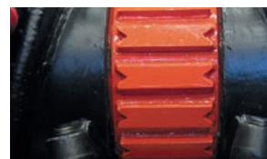
Hardox gear protection
