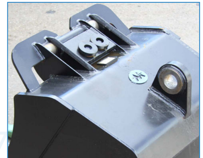
A-Lock 3 attachment-connection with spring bracket , wear compensation
