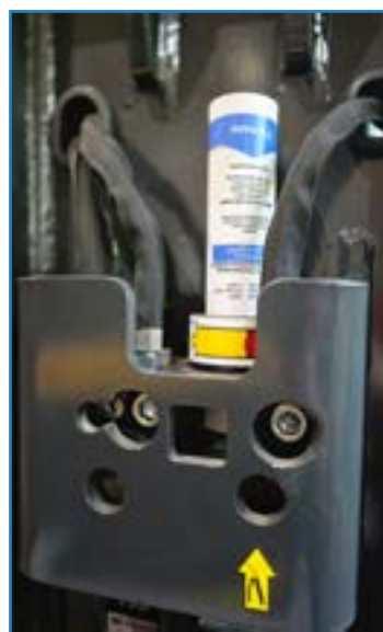
Central greasing pump - installation standard
