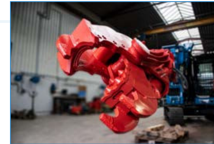
Demolition shear Tunn-CUT 500 H
