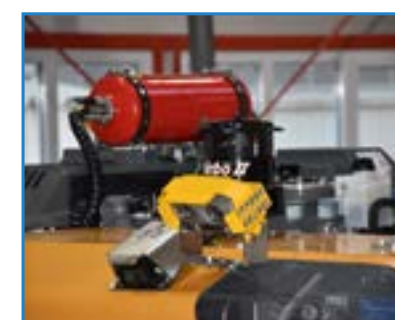
Extinguishing container and optional Blaxtair person detection system
