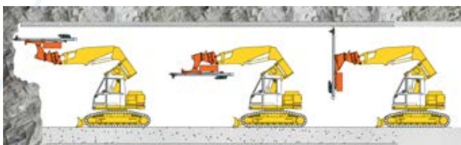
Movement options attachment-drilling-units with the T-model in the tunnel
