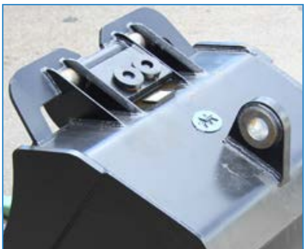
A-Lock 3 attachment-connection with spring bracket , wear compensation
