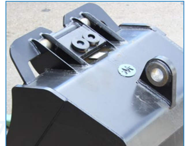
A-Lock 3 attachment-connection with spring bracket , wear compensation
